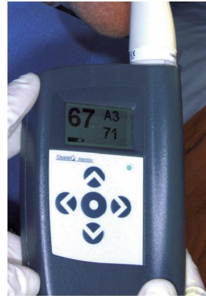
Fig. 14. In several implant systems, the Mentor™ gives one low and one high implant stability quotient value, reflecting the highest and the lowest level of stability of an implant.
