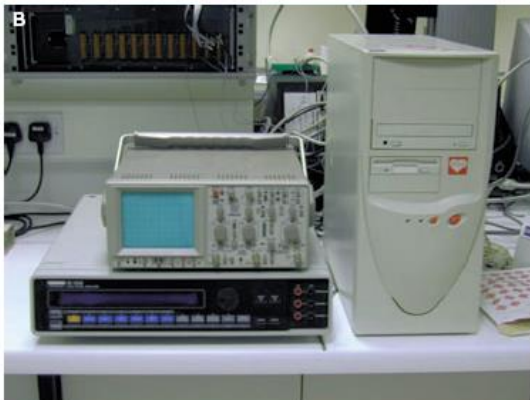
Fig. 7 (A) First-generation resonance frequency analysis transducer. (B) First-generation equipment, including a personal computer, an oscilloscope and a frequency response analyser.
